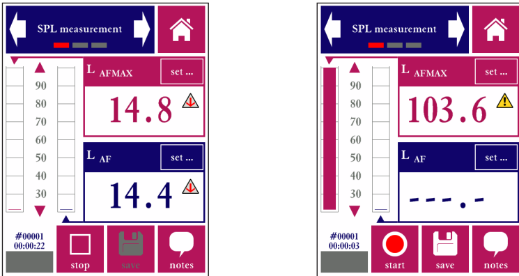
Range warnings are shown if the signal level is either too low or too high
